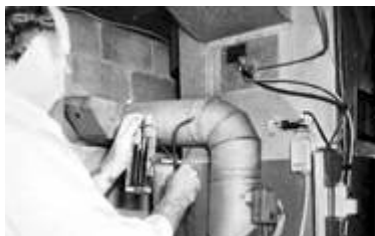
Taking a CO 2 reading with No. 1101 CO 2 indicator is quickly and easily done.
