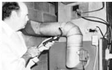
Taking a smoke sample with Dwyer Smoke Gage Pump and filter paper.
