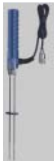
#202-30-E/C Used for bales, 9 1/2" insulated pins, with 8 1/4" penetration, eliminate the effect of surface moisture
